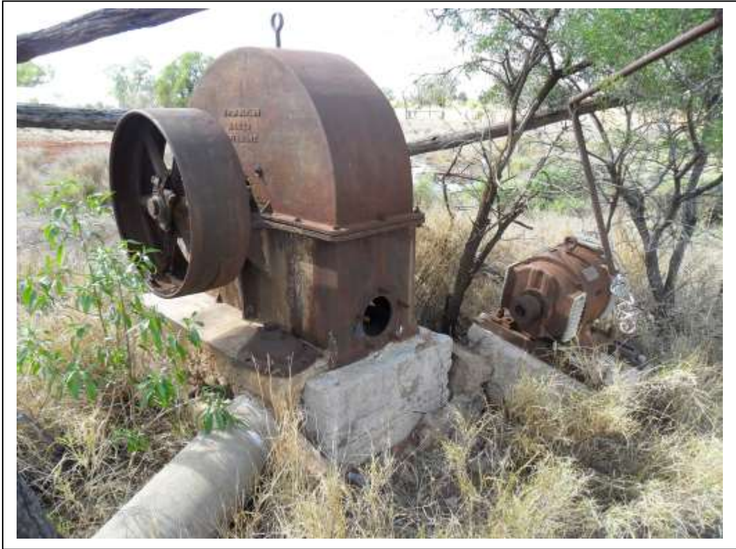
Pelton wheel and dynamo at Warrambah station, Cunnamulla district Queensland (Photo courtesy Bob Bird)
